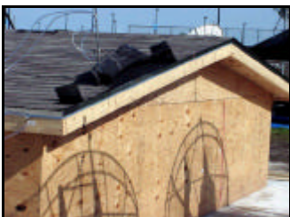
Left: (b) roof water penetration tests using air boats and a rain generator wind tunnel
