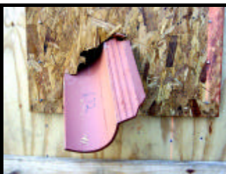
Left: (c) debris impact tests using a compressed air cannon
