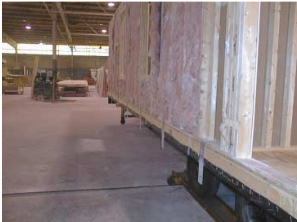
Tie-down connector attached to floor framing.
