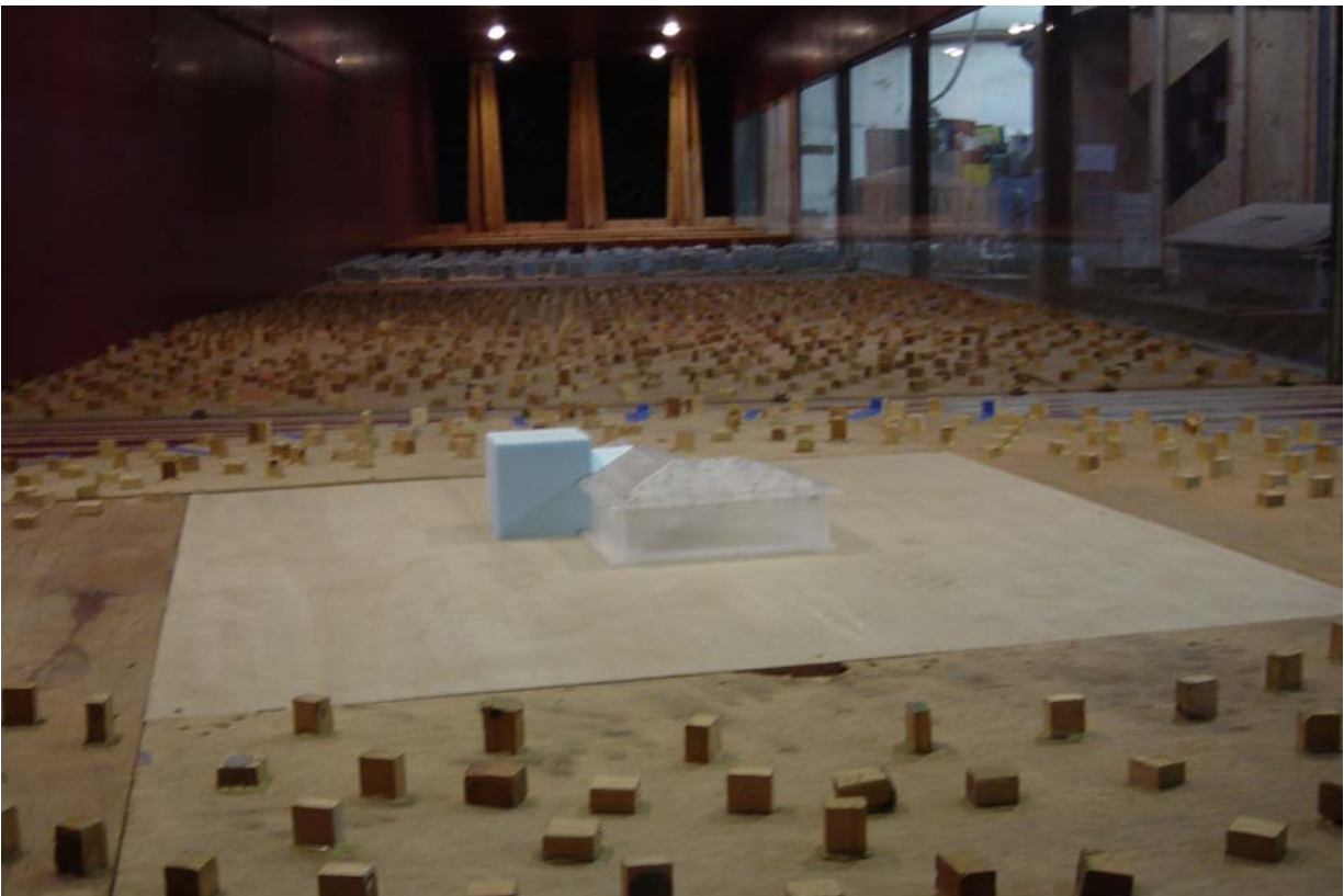
Figure 1. Photograph of One of the IHRC Models in the BLWT at Clemson University.
