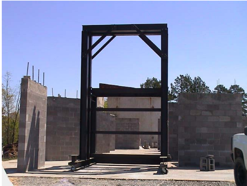
Figure 1. Bare Reaction Frame Supported on Steel Wheels for Movement to Test Specimen.
