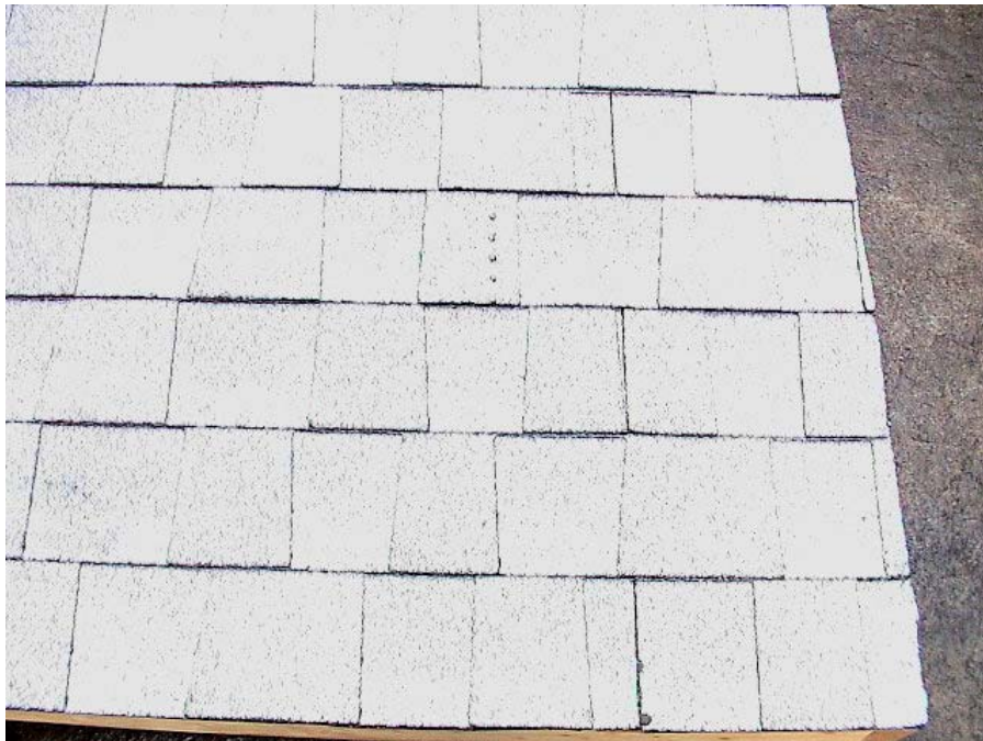
Figure 4. Photograph of Portion of Test Specimen with Pressure Taps.
