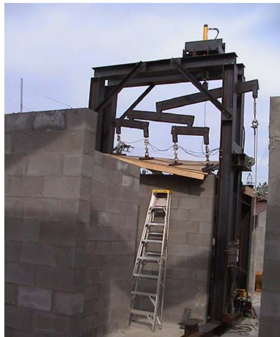
Figure 1. Bare Reaction Frame Supported on Steel Wheels for Movement to Test Specimen.
