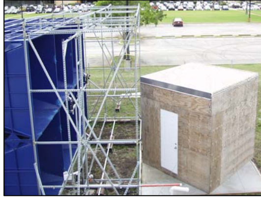
Figure 3. WOW Test Structure in Front of WOW at 45° angle
