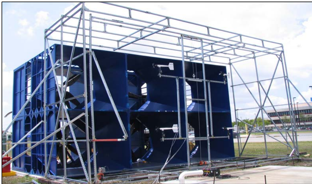
Figure 17. Unistrut Velocity Measuring Frame in Front of WOW
