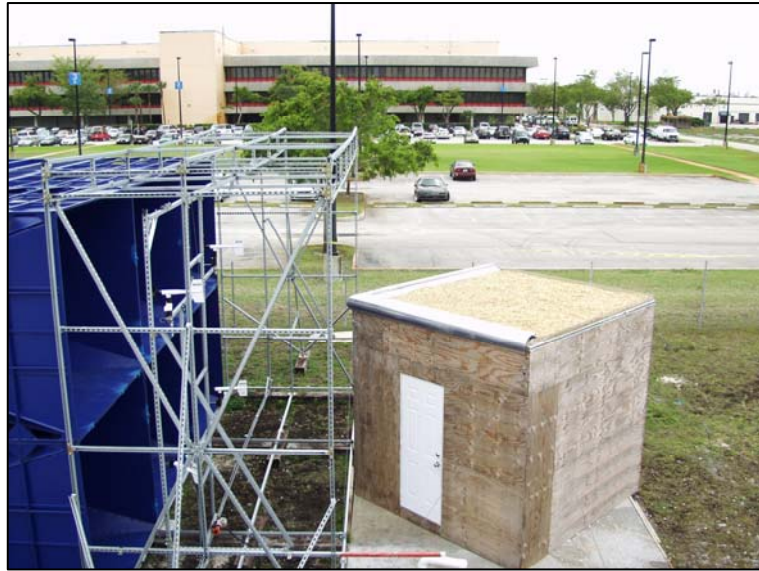
Figure 26. Test Structure Equipped with Flat Roof AeroEdge Cap
