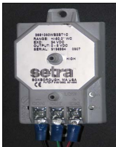
Figure 6. Setra Model 265 Very Low Differential Pressure Transducer
