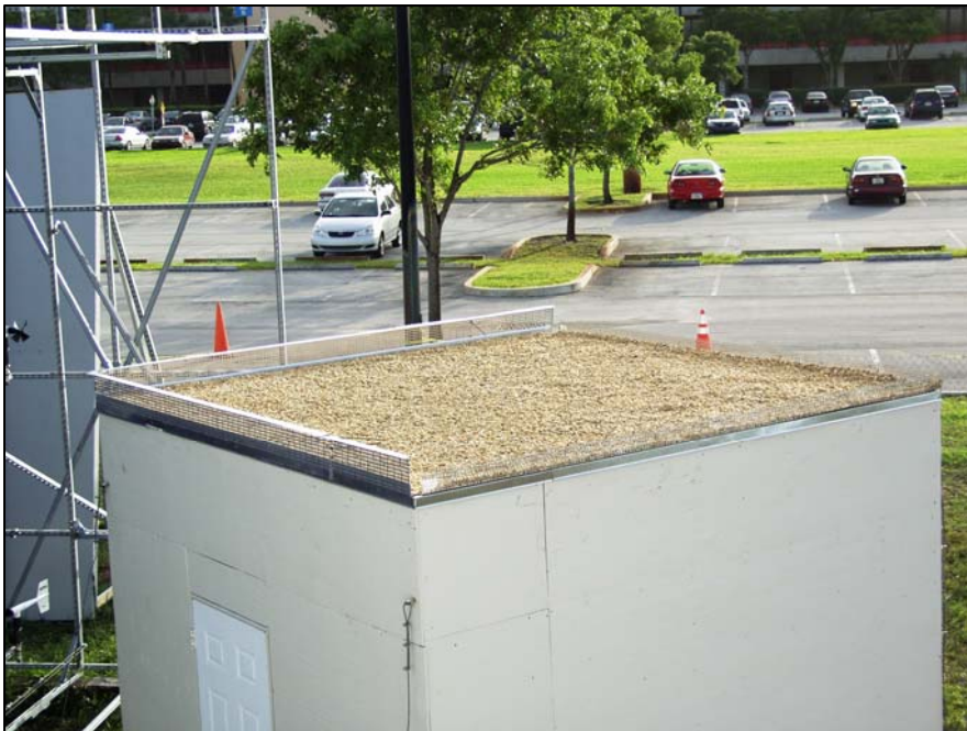
Figure 36. Gravel Scour Associated with FRAG1 edge shape at 4400 rpm
