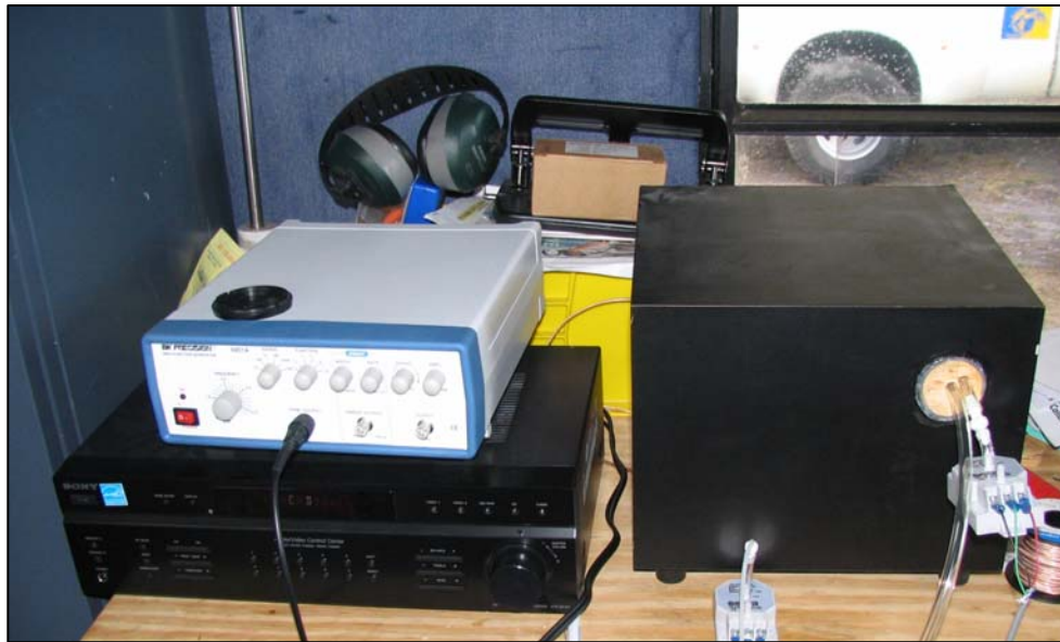
Figure 14. Set-up for Dynamic Calibration of Pressure Transducers
