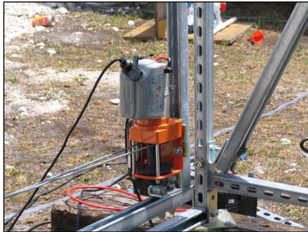
Figure 19. Close-up Winch used to Move Unistrut Frame Up and Down and Side-to-Side
