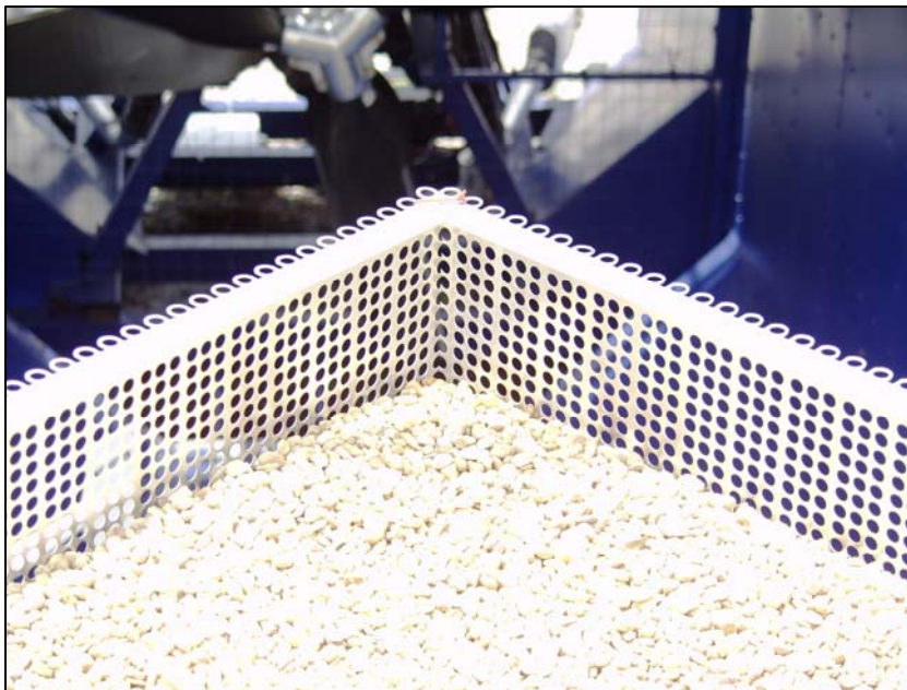
Figure 33. Gravel Scour Associated with FRAG1 AeroEdge™ Shape at 3000 rpm
