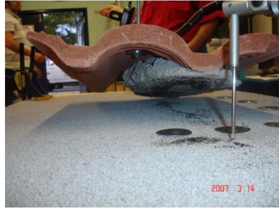
Figure 3.19: Typical Failure Surface of Concrete Tile with Mortar-Set
