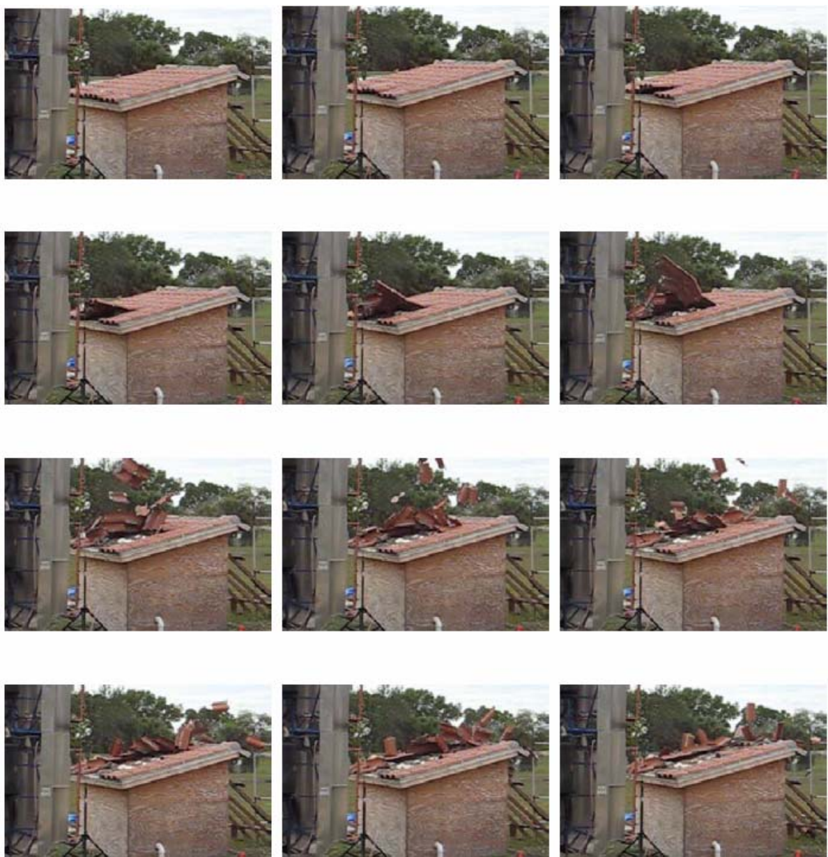
Figure 5.23: Failure Progress of Clay-with-Mortar Tile Roof System (120 mph Wind Speed at 0° Direction)
