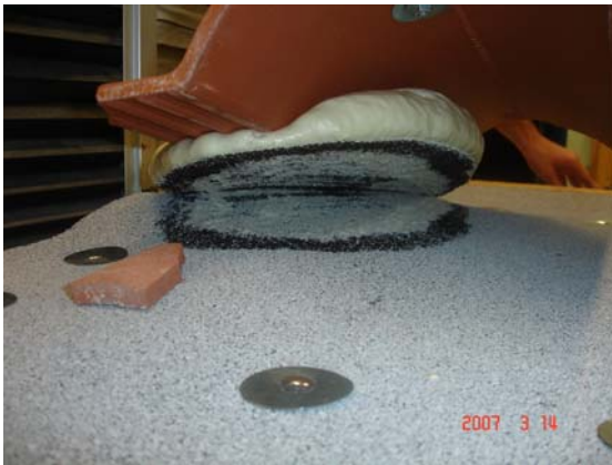
Figure 3.16: Typical Failure Surface of Clay Tiles with Adhesive-Set
