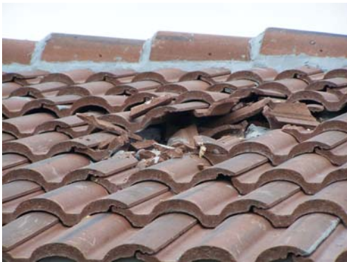
Figure 4.5: Impact Test on Concrete with Mortar Tile Roof System
