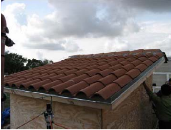
(a) Model 1a: Clay Roof Tiles with Foam
