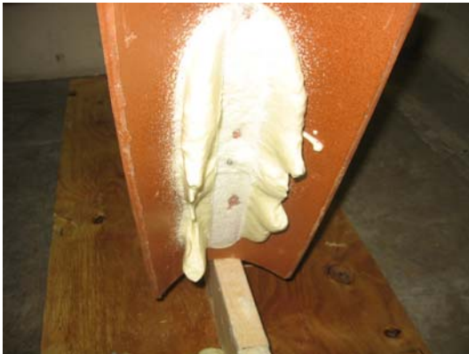
Figure 3.6: Typical Failure Surface of Adhesive-Set with Clay Tile
