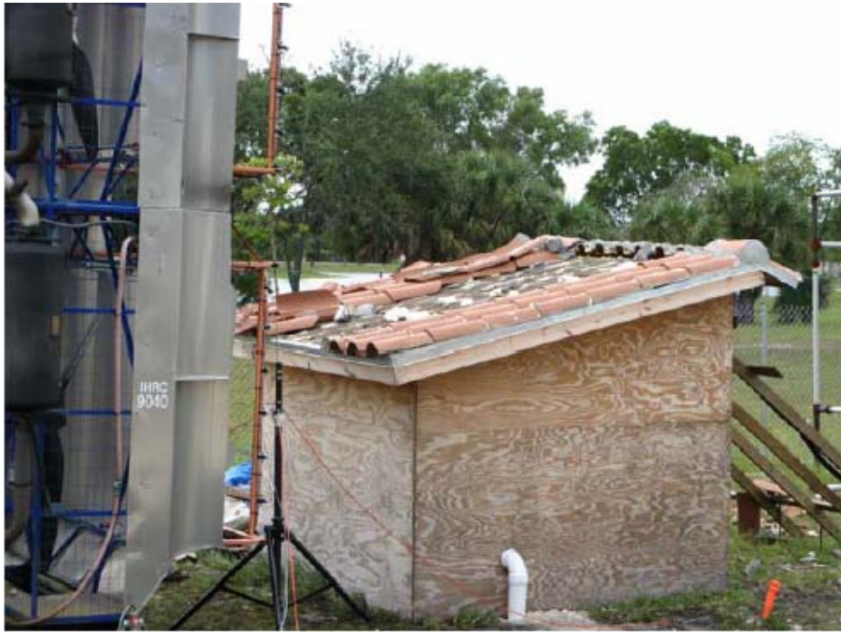
(a) Roof Conditions Subjected to 120 mph Wind Speed at 0^{\circ} Direction
