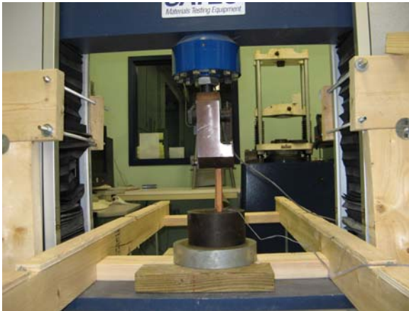
Figure 6.1: Clay Tile Strip under Axial Compression
