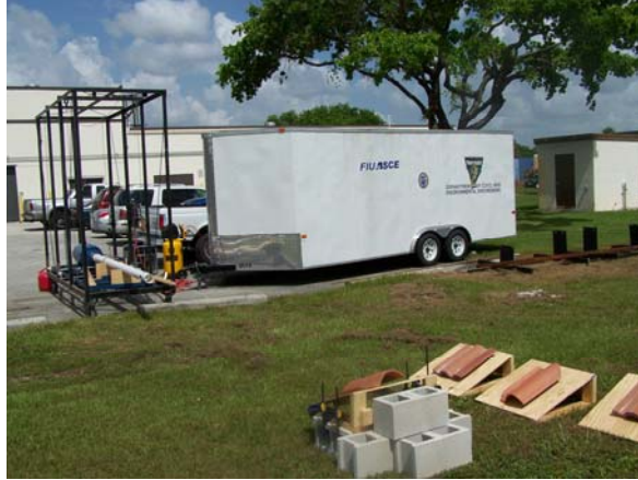
Figure 4.2: Air Cannon Impact Test for Single Field Tiles
