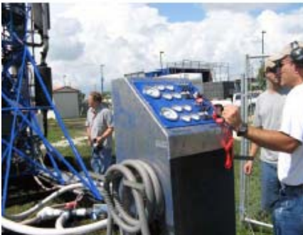
Figure 5.2: 2-Fan WoW Control System
