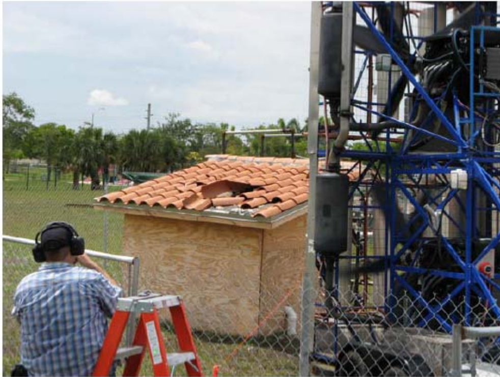
(a) Roof Condition Subjected to 120 mph Wind Speed at 0° Direction
