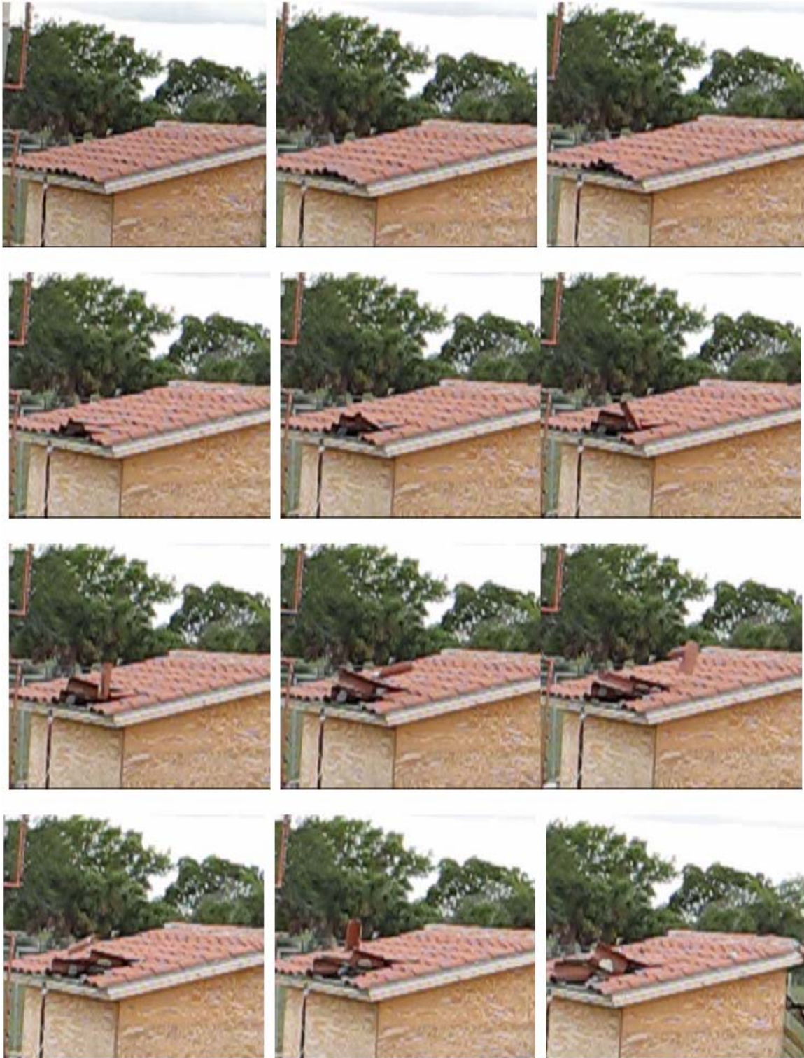
Figure 5.16: Failure Progress of Clay-with-Foam Tile Roof System (120 mph Wind Speed at 0° Direction)
