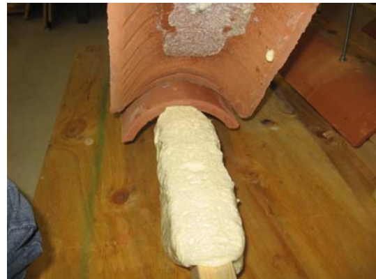
Figure 3.7: Typical Failure Surface of Adhesive-Set with Concrete Tile
