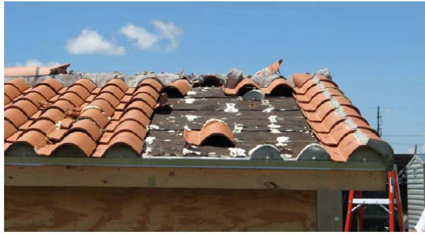
(a) Roof Conditions Subjected to 120 mph Wind Speed at 0° Direction
