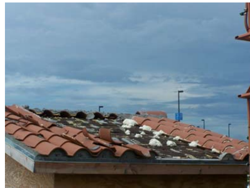
Figure 4.6: Impact Test on Clay with Foam Tile Roof System
