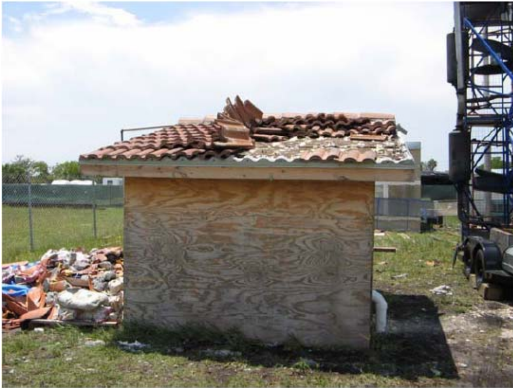
(a) Roof Conditions Subjected to 120 mph Wind Speed at 50^{\circ} Direction
