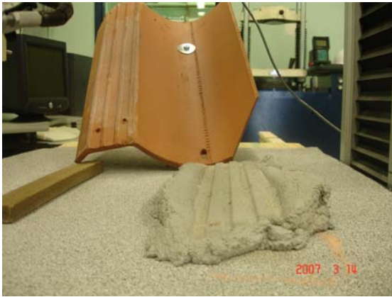
Figure 3.18: Typical Failure Surface of Clay Tile with Mortar-Set
