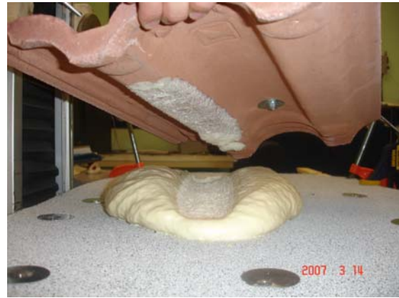
Figure 3.17: Typical Failure Surface of Concrete Tiles with Adhesive-Set
