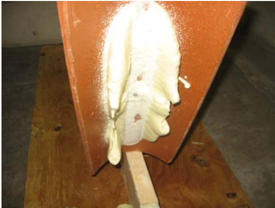
Figure 3.4: Typical Failure Surface of Adhesive-Set with Clay Tile
