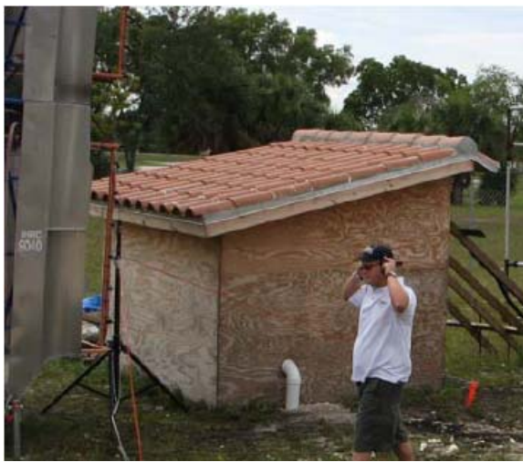
(c) Model 2: Clay Roof Tiles with Mortar
