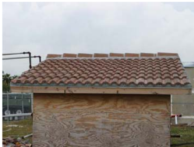
(e) Model 4: Concrete Roof Tiles with Mortar
