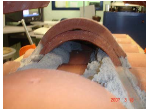
Figure 3.10: Typical Failure Mode of Concrete Tiles with Mortar-Set
