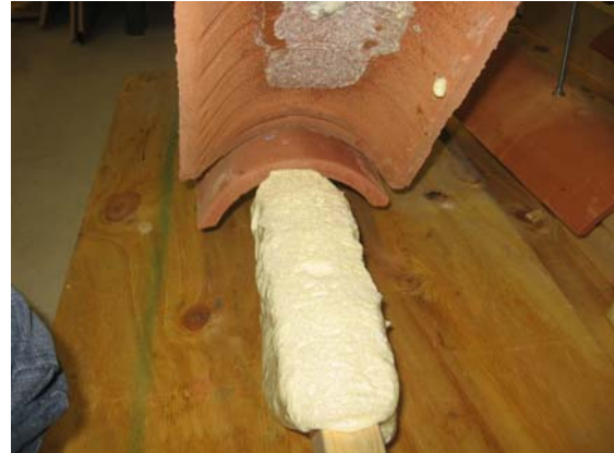
Figure 3.5: Typical Failure Surface of Adhesive-Set with Concrete Tile
