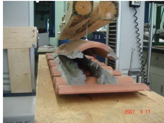
Figure 3.12: Typical Failure Mode of Concrete Tiles with Mortar-Set
