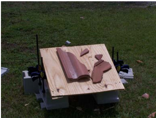
Figure 4.3: Single Concrete Field Tile After Projectile Impact
