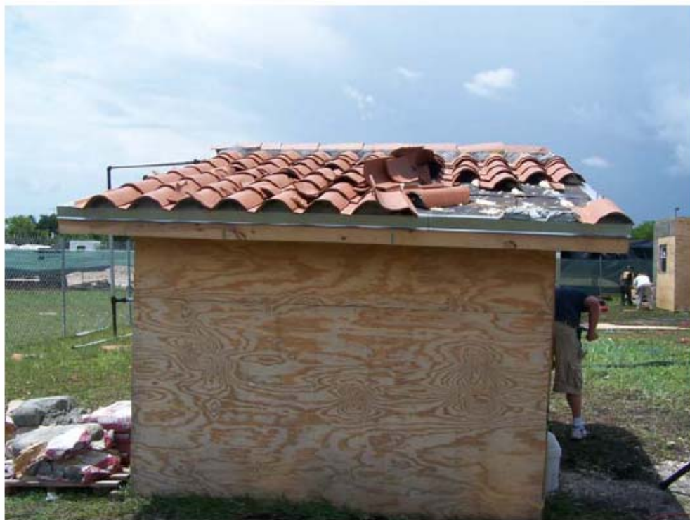
(b) Roof Condition Subjected to 120 mph Wind Speed at 50° Direction
