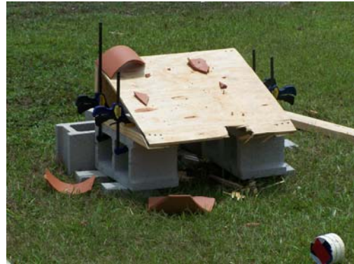
Figure 4.4: Single Clay Field Tile After Projectile Impact
