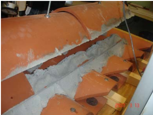
Figure 3.9: Typical Failure Mode of Clay Tiles with Mortar-Set
