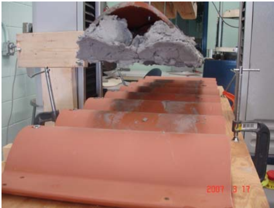
Figure 3.11: Typical Failure Mode of Clay Tiles with Mortar-Set
