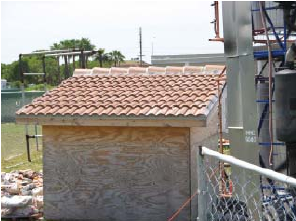
Figure 5.29: Concrete-with-Mortar Tile Roof System after Wind Testing
