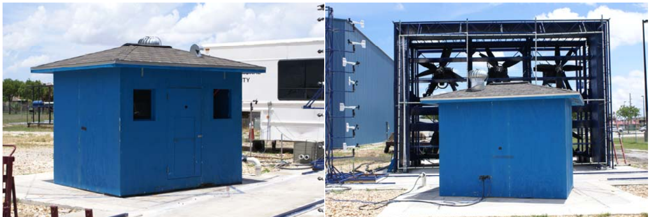
Figure 28: Wooden hip roof model in front of Wall of Wind
