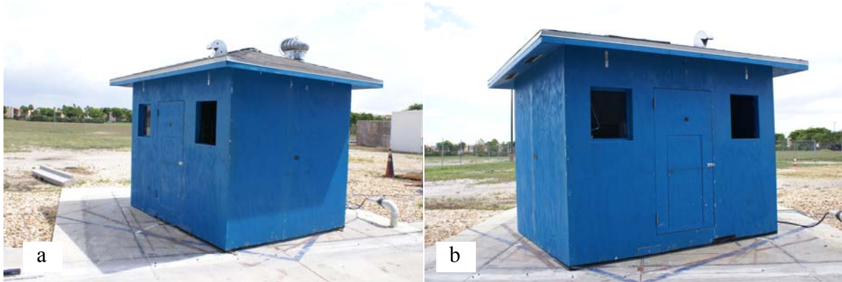
Figure 50: Hip roof model for Test case 3: a) at 15° and b) at 120° wind angle of attack (only right side window open)
