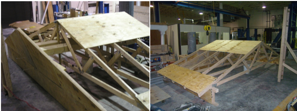
Figure 4. Test Setup with Semi-Covered and Fully-Covered Sheathing.
