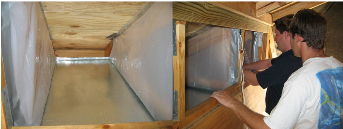
Figure 14 A Poor Choice for Wetting Measurements: Drip Pans
