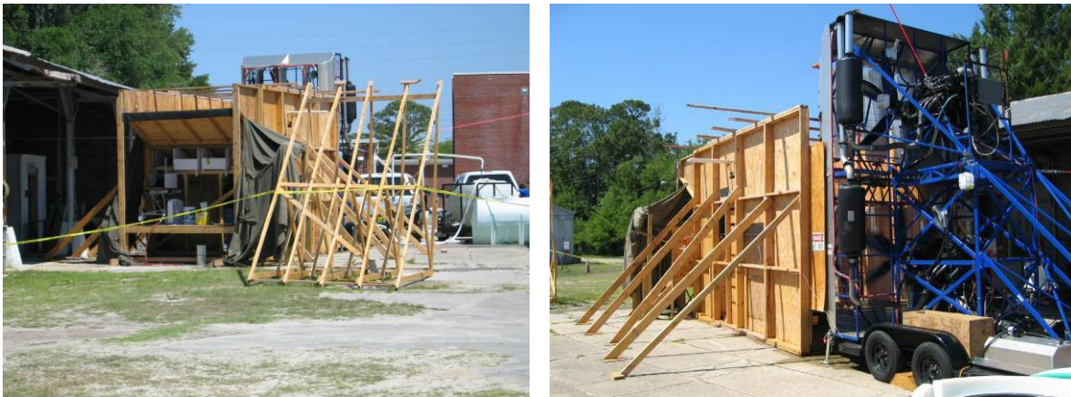
Figure 5 Final Wall of Wind Configuration
