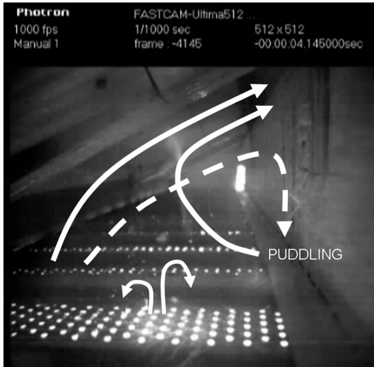
Figure 8 Typical Primary and Secondary Raindrop Paths
