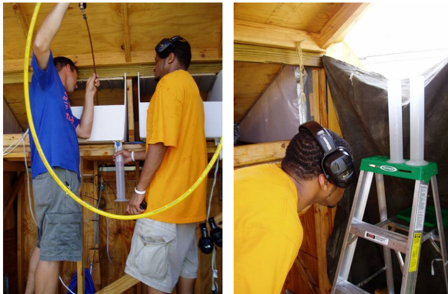
Figure X Measurement of Water in Catch Basins
